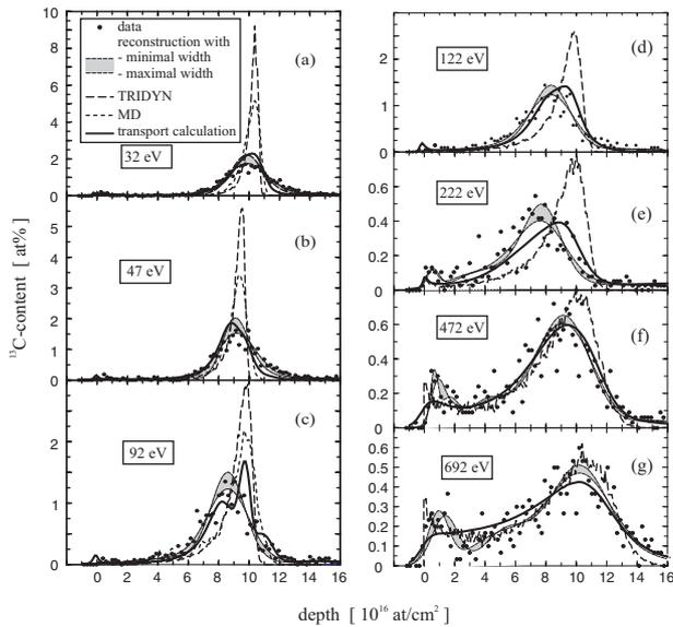
Fig. 2: Measured and calculated  $^{13}\text{C}$  mixing distributions at ion energies which are shown in the plot. TRIDYN and transport calculations are carried out for a  $9 \times 10^{16}$  at/cm $^2$  thick  $^{12}\text{C}$  cap layer. The MD simulation is performed for ion energies  $E_{\text{ion}} \leq 92$  eV and a  $5 \times 10^{16}$  at/cm $^2$  thick  $^{12}\text{C}$  cap layer due to the high CPU time consumption.
