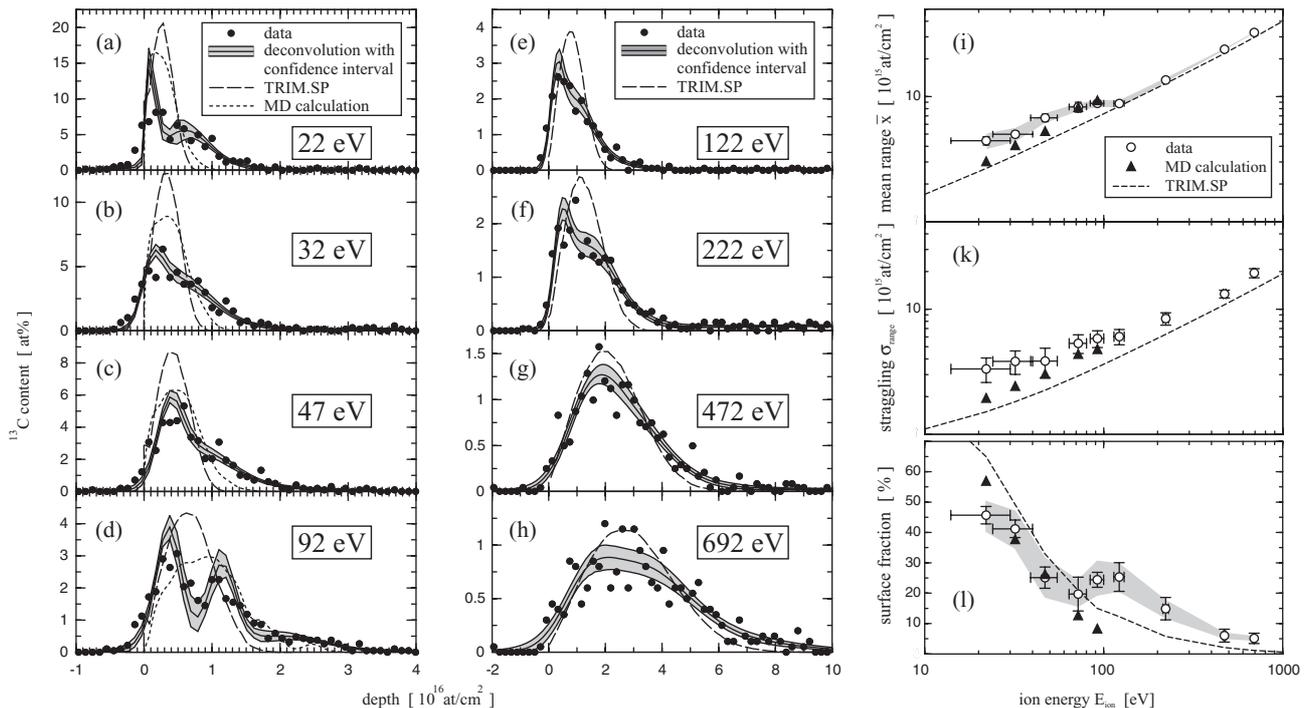
Fig. 1: (a)–(h) Measured and calculated range distributions of  $^{13}\text{C}^+$  ions implanted at energies which are shown in the plot. The substrates are amorphous  $^{12}\text{C}$  layers grown by mass-selected ion-beam deposition (MSIBD) at the same energies, respectively. (i) Measured and calculated mean ion ranges, (k) range straggling and (l) fraction of  $^{13}\text{C}^+$  ions incorporated within the topmost  $3 \times 10^{15}$  at/cm $^2$ .
