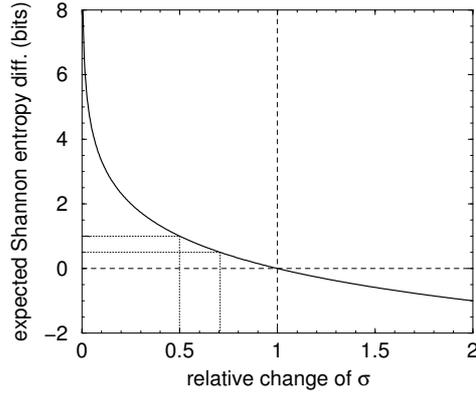
**FIGURE 1.** Expected Shannon entropy difference as a function of the relative change of the standard deviation of a mean estimate
