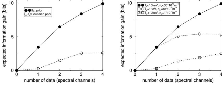
**FIGURE 3.** Expected information gain in units of bits as a function of the number of spectral channels used to measure the Thomson scattering light. Left: The full circles (open circles) depict the expected information gain for a prior distribution constant in the full parameter range (Gaussian in a small parameter space), respectively. Right: Decomposition of the information gain assuming either  $T_e$  (open circles) or  $n_e$  (open squares) to be known exactly.
