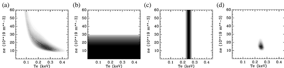
**Fig. 3.** Integrated Data Analysis: The combination of PDFs from different diagnostics for a single spatial position. (a) is the Thomson scattering result (b) indicates operation of a microwave interferometer, (c) is a temperature measurement from soft X ray measurements. Panel (d) is the combination of the (a-c).
