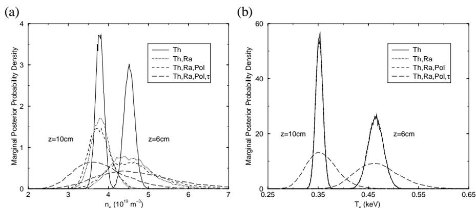
**Fig. 2.** Marginal posterior PDF for the density measurement (a) and the temperature measurement (b) of two spatial channels ( $z = 6 \text{ cm}$  and  $z = 10 \text{ cm}$ ) of the Thomson scattering system under consideration. Here, different nuisance parameters are switched on subsequently.
