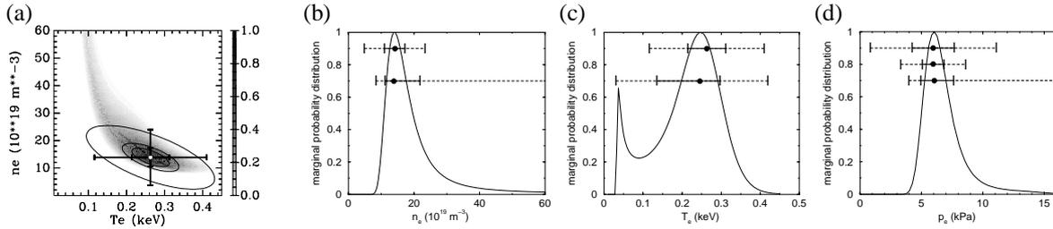
**Fig. 1.** Marginal posterior PDF (the probability is encoded by the gray scale) representing the result of a Thomson scattering system (a), for details see section 3. Figs. (b) and (c) show the projection of (a) onto the corresponding axes. (d) shows the marginal posterior PDF for a derived quantity, namely the electron pressure. For details of the different error bars see Ref. [3].
