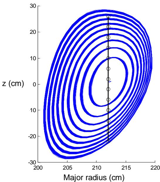
Fig. 5 Uncertainty of magnetic mapping. Thomson scattering line of sight superimposed.
