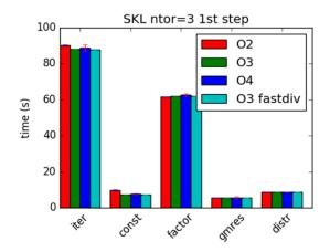
Fig. 2 Execution times using different compiler flags
