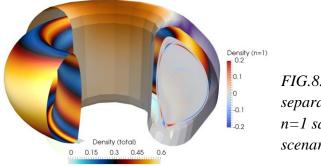
FIG.8.(a) 3-D density structure at the separatrix and resistive wall potential of a n=1 saturated kink mode in ITER Q=10scenario
