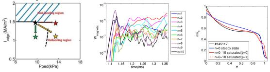
FIG. 4. (a) Sketch of the stability diagram of the equilibria studied with a range of edge current and pedestal pressure levels; (b)Perturbed magnetic energy evolution of n=1-10 modes for the JOREK simulations with increased pressure at pedestal; (c) Density profiles for n = [0-10] during saturation phase at t=1.35ms.
