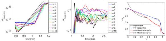
FIG. 3. Time evolution of the perturbed magnetic energy of each harmonic for n=1-10 modes at linear growth phase(a) and at saturation phase(b) for the JOREK simulations; (c) Density profiles for n = [0-10] at saturation phase.
