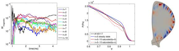
FIG.6. JOREK simulations including n=0-10 modes with the reduced edge current and higher pedestal pressure equilibrium. (a) Time evolution of the magnetic energy during saturated phase; (b) pressure profiles for n = [0-10] in saturated phase (c) contour plot of the poloidal flux perturbation in saturated phase with separatrix(black curve).
