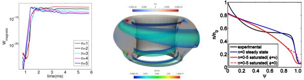
FIG. 1. (a)Time evolution of the perturbed magnetic energy of each harmonic for n=1-5 kink peeling mode from the JOREK simulation; (b) 3-D helical structure of the density perturbation for a saturated n=1-5 KPM at separatrix; (c) density profiles for an n = [0-5] saturated KPM.
