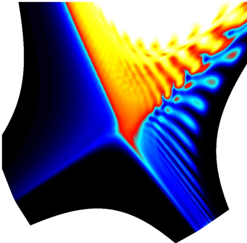
*Detached filaments quickly lose their pressure due to fast parallel heat conduction. Substructures appear in divertor heat flux patterns.*
