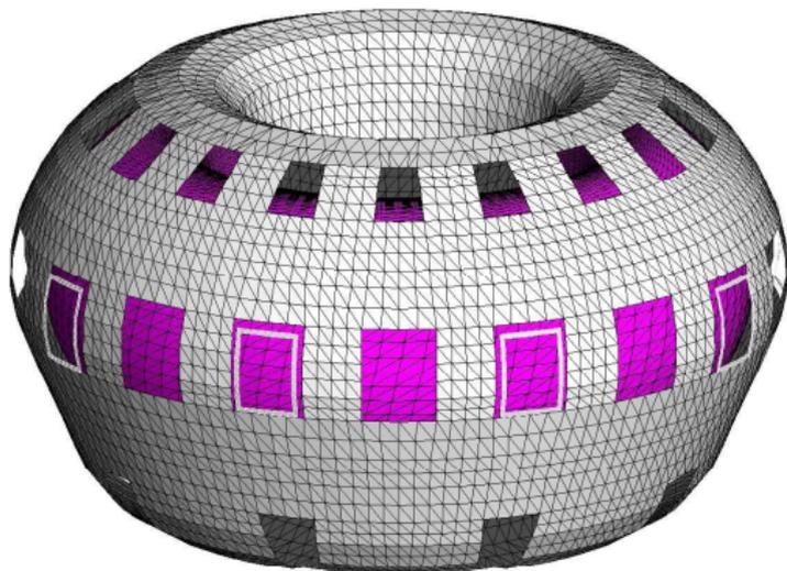
*Discretization of first ITER wall in the STARWALL code which describes vacuum region and wall currents*
