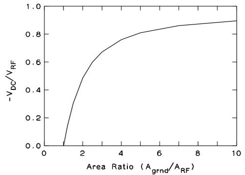
**Figure 9.** The ratio of the bias and the RF voltage against the area ratio, for a driving voltage  $eV_{RF} = 120 kT_e$ . The frequency is 13.56 MHz.
