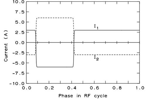
**Figure 6.** The total current to each electrode for the potential curves of figure 5. Here only one cycle is shown.
