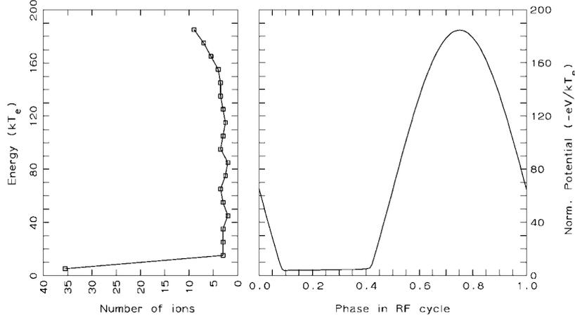
**Figure 11.** The ion energy distribution at low frequencies.
