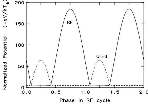
**Figure 5.** The normalized potential drop over the space charge sheaths in an RF discharge in argon ( $M_+ = 40$ ), with an area ratio  $\alpha = 2$ , at a frequency of 100 kHz. The normalized RF voltage and dc bias are 120 and 59.7, respectively. Note that two cycles are shown.
