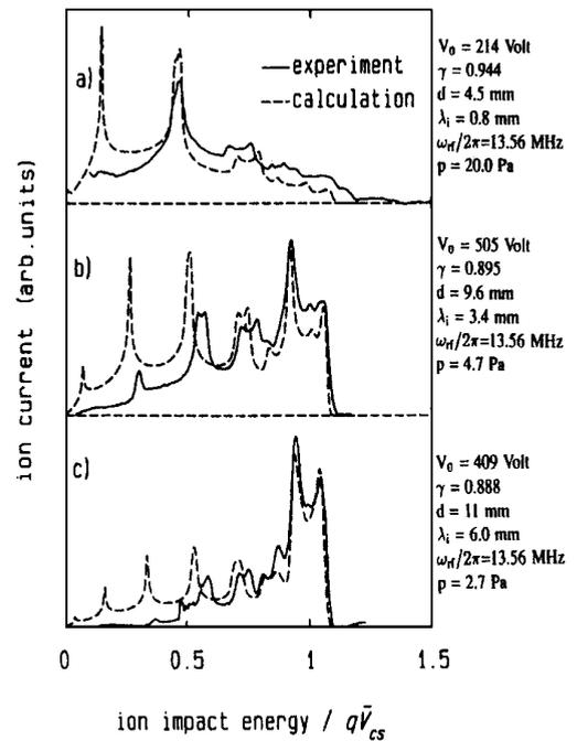
**Figure 14.** Examples of experimentally and numerically obtained ion energy distributions at the powered electrode. The relevant parameters are given at the right-hand side of each plot. Illustration from [12].
