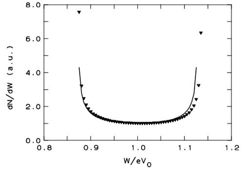
**Figure 12.** The ion energy distribution at high frequencies. The parameters are a frequency of 15 MHz, a modulation factor of 0.95, an amplitude of 500 V, a mass of  $40 M_H$  and a sheath width of 5 mm. The full curve is the approximation and the symbols are computed without neglect of small terms.
