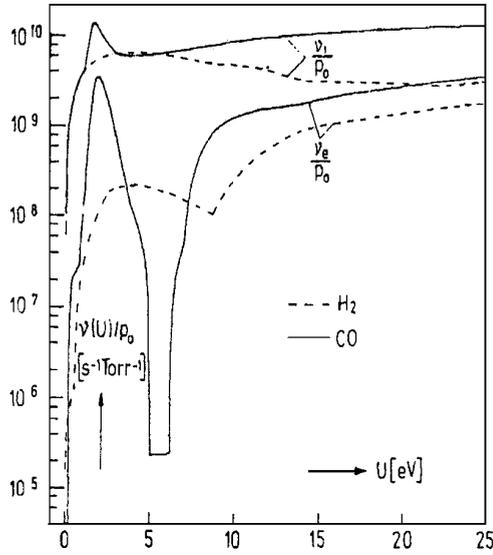
**Figure 15.** The frequency of the loss of momentum and the energy of electrons in a molecular gas. Note that the energy loss is almost totally covered by the inelastic processes. Illustration from [14].
