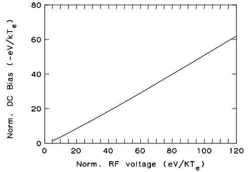
**Figure 8.** Bias against RF voltage for an area ratio  $\alpha = 2$ . The frequency is 13.56 MHz.
