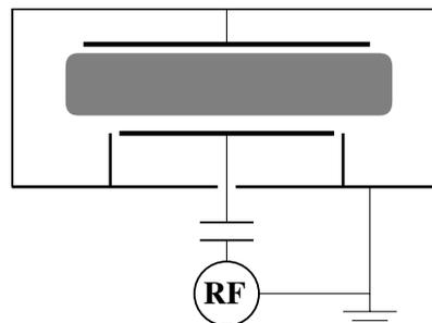
**Figure 1.** Schematic diagram of the geometry of a planar RF discharge; not drawn are the gas inlet and the vacuum pumps.
