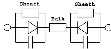
**Figure 10.** Equivalent circuit of a RF discharge.
