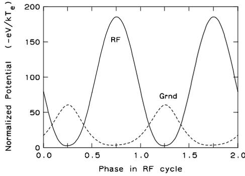
**Figure 7.** As figure 5, but for a frequency of 13.56 MHz. The normalized dc bias is 62.0.
