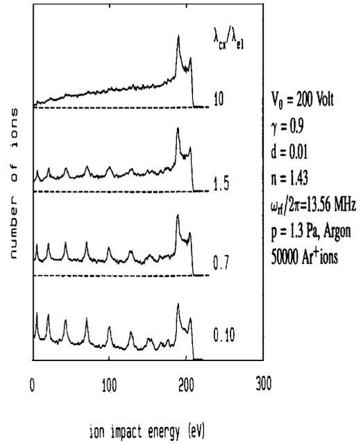
**Figure 13.** Changes in the ion energy distribution function when the relative contribution of elastic collisions is changed from ten times (top) to one tenth (bottom) of that of the charge exchange. The distributions are obtained from a Monte Carlo calculation for a sheath with parameters given at the right-hand side. Illustration from [11].
