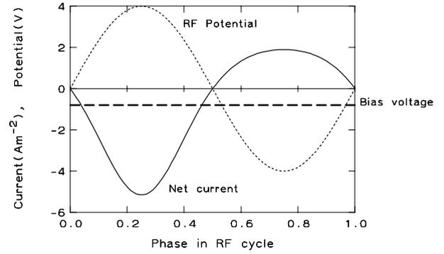
**Figure 3.** Current against phase of an RF signal applied to a floating probe. Current equilibrium can only be reached by the generation of an extra bias voltage.
