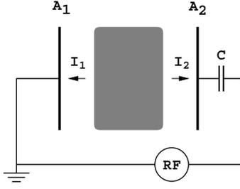
**Figure 4.** The RF discharge as a system of two planar probes.
