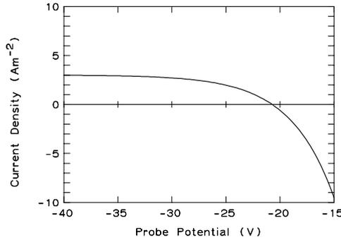
**Figure 2.** A current–voltage characteristic for a planar probe in a Maxwellian plasma with  $N_\infty = 10^{16} \text{ m}^{-3}$ ,  $M_+ = 40M_H$ , and  $kT_e = 4 \text{ eV}$ .
