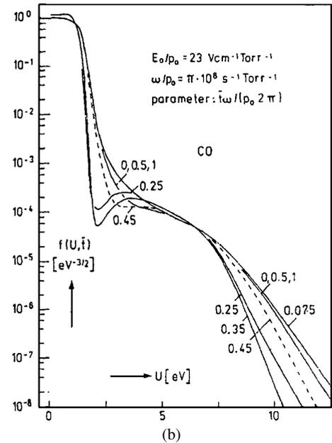
**Figure 16.** Electron energy distribution in a molecular gas at various phases of the RF cycle, for a low (a) and a high (b) RF frequency. Illustration from [14].
