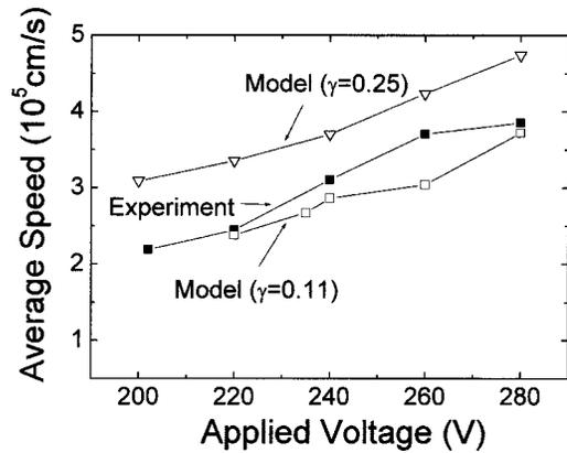
FIG. 7. Measured and calculated plasma expansion (or sheath contraction) velocity as a function of the applied voltage pulse amplitude (pure neon, 5 Torr, geometry of Fig. 2).
