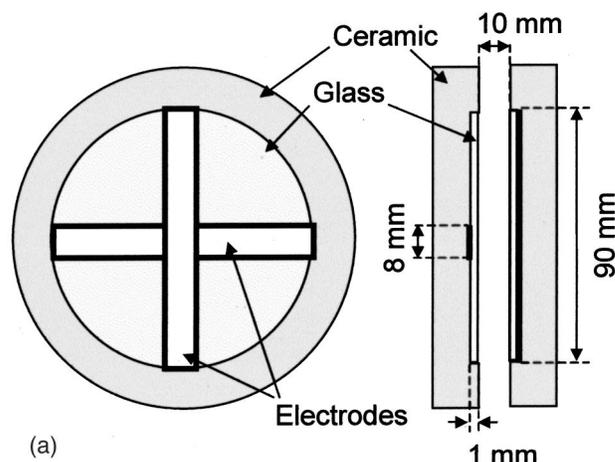
FIG. 2. (a) Electrode structure and applied voltage wave form. (b) Simulation domain is 2D cartesian (i.e., the discharge is supposed to be infinite and uniform along the direction perpendicular to the simulation domain). Vertical electrode is, therefore, equivalent to a plane in the 2D simulation.
