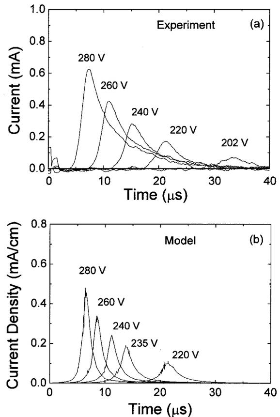
FIG. 4. (a) Measured current pulses for different voltage amplitudes (conditions of Fig. 3). (b) Calculated current pulses for different voltage amplitudes (conditions of Fig. 3).
