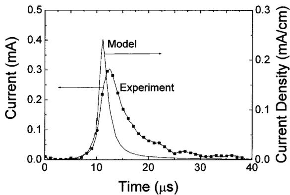
FIG. 3. Measured (symbols) and calculated current pulses in pure neon, 5 Torr, for a 1 cm gap length for the geometry and dimensions of Fig. 2 (standard case). Voltage pulse amplitude is 240 V and the voltage frequency is 150 Hz. Units for the model results are in milliamperes/centimeters (right-hand side axis). The capacitive current during the rise and decay of the voltage pulse has been subtracted from the measured and calculated total current.
