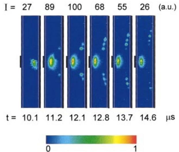
FIG. 5. (Color) ICCD side view images of the plasma at different times when the vertical electrode is the anode in the geometry of Fig. 2 in pure neon, 5 Torr. The amplitude and frequency of the voltages are 245 V and 150 Hz, respectively.
