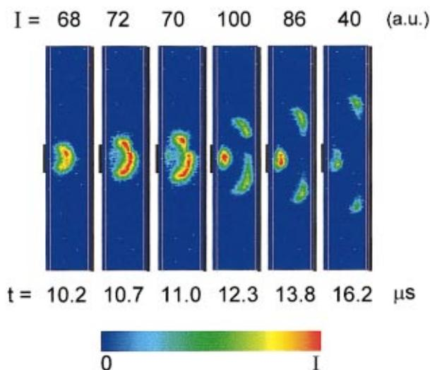
FIG. 8. (Color) ICCD side view images of the plasma at different times when the vertical electrode is the cathode in the same conditions as Fig. 5.
